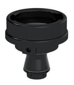
This solution is suited for tank necks which are sheltered by very low decks or within limited, confined spaces. It is a versatile solution featuring a swinging body which allows refueling pistol insertion at angles which may avoid collision between the pistol and surrounding structures.
